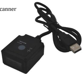
The RT235 is a new generation scanner launched in 2020. It's outstanding at its super small & compact design, lower power consumption and ability to read even poor quality bar codes and reading from phone screen even when the screen is lower brightness.
