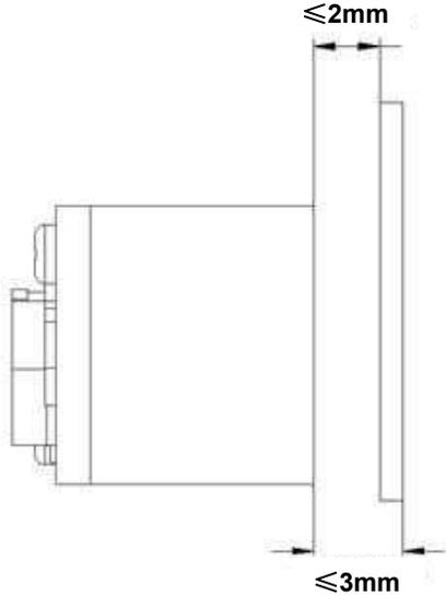
If the window is required to be in a tilted position, the above distance requirements should be met and tilt angle should ensure no reflections back into the lens.
