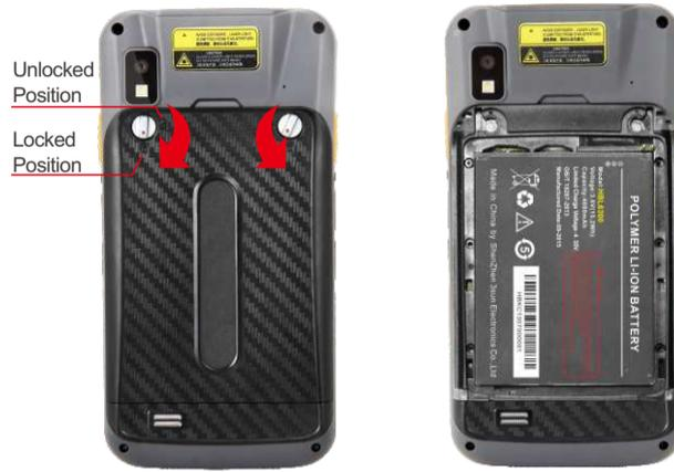
Note: Gently rotate the battery cover clip in quarter-turn motion. Do not apply excessive force.
