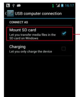
Check this to enable device as a USB storage to PC.
