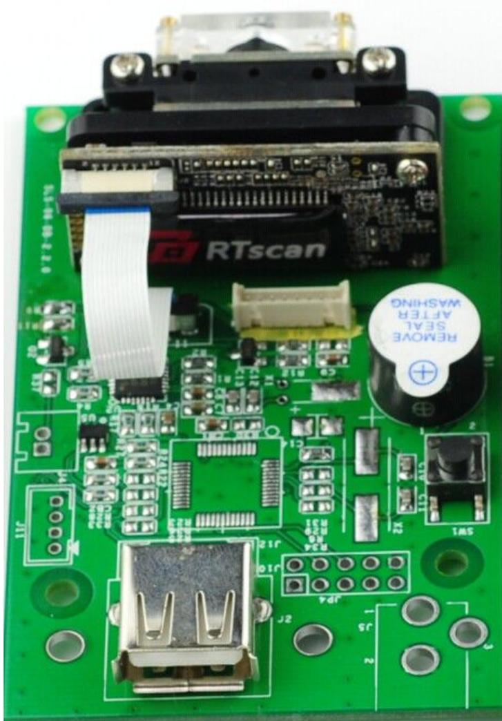
RTscan provides a emulation Kit with USB interface, fix the barcode scan engine RT200 in the emulation Kit ,and connect the emulation Kit (together with the RT200) to your system via USB cable.
