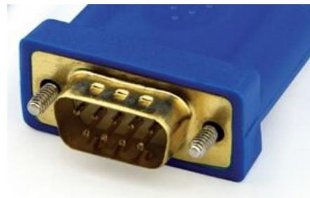
RTscan provides a emulation Kit with 9 PINs RS232 interface, fix the barcode scan engine RT200 in the emulation Kit , and connect the emulation Kit (together with the RT200) to your system via RS232 cable.
