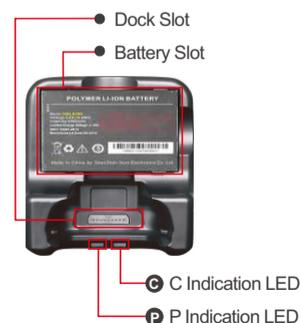
When starts to charge battery, the P indication LED of dock will be green. The red C indication LED will turn green after battery is fully charged.
