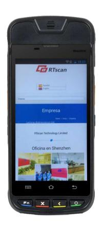
RT940 is a "PDA + POS" all in one Android smart pos computer, It combines the functions of financial POS and Android PDA, with 5 inch large touch screen, MSR reader, contact and contactless IC card reader, thermal printer, barcode reader, WI-FI, Bluetooth, 3G, GPS, support traditional payment, NFC payment and barcode payment.
