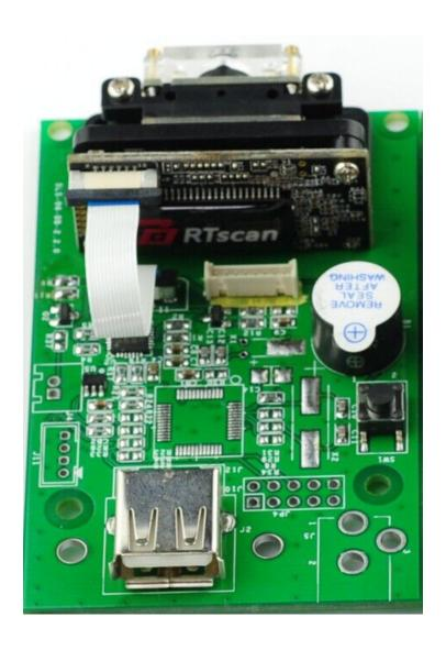
RTscan provides a emulation Kit with USB interface, fix the barcode scan engine RT200 in the emulation Kit ,and connect the emulation Kit (together with the RT200) to your system via USB cable.
