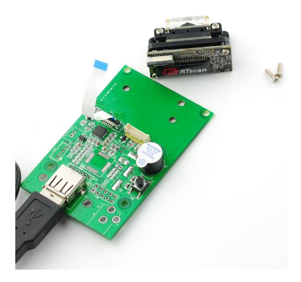
Same as USB-VCOM that need to use a emulation Kit which with USB interface, and the scan engine RT200 fixed in this emulation Kit, and you connect the emulation Kit (together with the RT200) to your system via USB cable.
